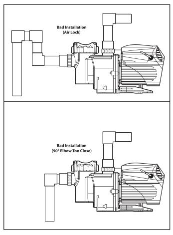
Figure 5. Viron XT Pump Incorrect Piping Installations
