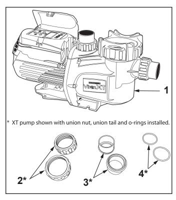
Figure 3. Viron XT Pump Components
