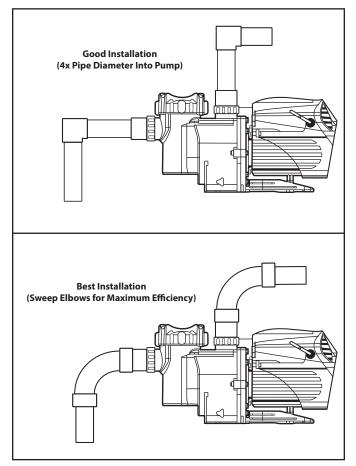
Figure 6. Viron XT Pump Good Piping Installations
