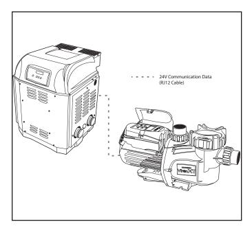
Figure 16. Viron XT Pump with RJ12 Cable Connection
