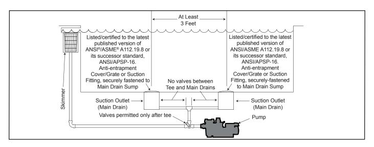
Figure 9. Number of Suction Outlets Per Pump
