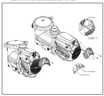
Figure 10. Data Port Location on XT Pump
