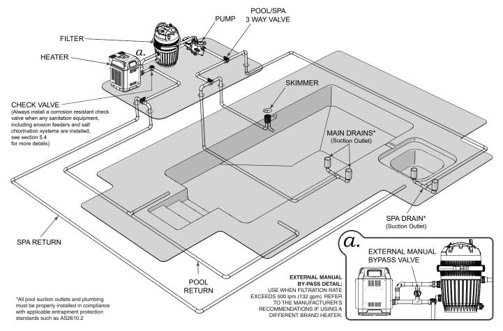
Figure 8. Typical Water Piping Configuration
