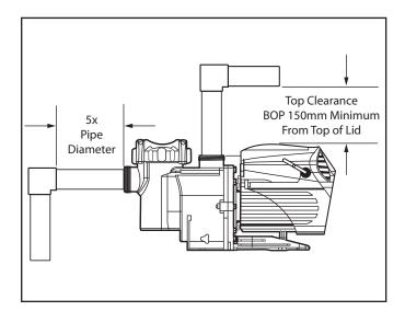
Figure 7. Viron XT Pump Piping Clearance
